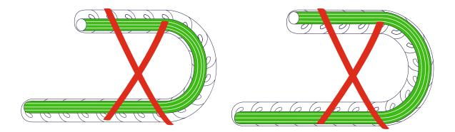
In the case of linear as well as horizontal traverse, round electrical conductors and pneumatic tubes must be fastened on both sides immediately following the drag chain in such a way as to relieve tension.
