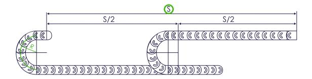
An important factor in fulfilling the expected lifetime of a cable is maintaining the maximum travel distance of the application. Information on the maximum travel distance can be found on the respective data sheet of the cable.
