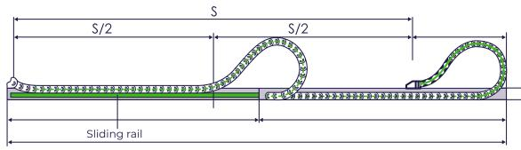
A bending cycle is usually a completed travel of the application from the start to the end position, i.e. back and forth. The lifetime is described by the number of bending cycles.
