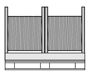
When delivering to our location in NL-Benthuizen, it is permitted to deliver 800 mm drums stacked twice on top of each other on one-way pallets (size 800 x 800 mm).
