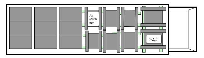
Drums (from size 900mm) up to 2.5 tonnes must be loaded transversely to the direction of travel, drums over 2.5 tonnes must be loaded lengthwise to the direction of travel and be ready to be unloaded from the side. In this case, it is absolutely necessary to notify us of the weight!
