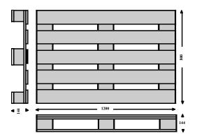
Euro pallet (pool pallet DIN 15 146, sheet 2, standard dimension and DIN 15 147, UIC 435-2 - NEW or class A).
